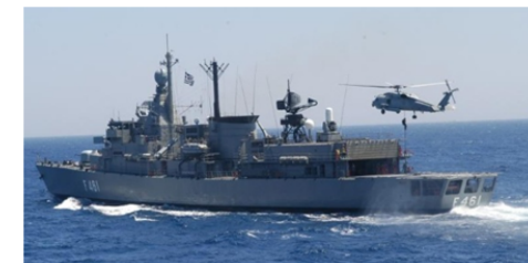
Figure 2-1. Asset Support – A helicopter controller on board the ship can direct a non-organic helicopter to a position near the flight deck. This enables the helicopter pilot to drop off people without landing the helicopter.
